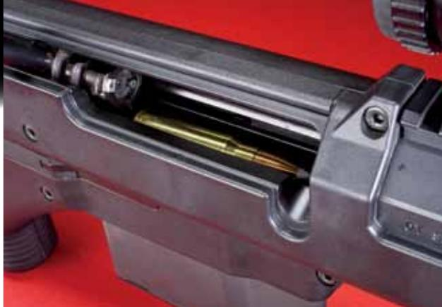
**Ammunition feeds from a detachable, single-stack magazine. When cycling the bolt, it only has to travel 4¼ inches to be ready to strip another round from the magazine and guide it into the chamber.**
