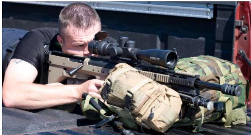
Florence, AL SWAT sharpshooter test fires the SRS .338 from pickup truck bed. SRS is sub- $\frac{1}{2}$ -MOA accurate with both .308 and .338 barrels using Black Hills ammo.
