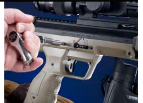
**Once new barrel is inserted, retaining bolts are re-tightened and torqued to 65 inch-pounds. Seekonk preset T Handled torque wrench from Brownells makes precise torque a "snap."**
