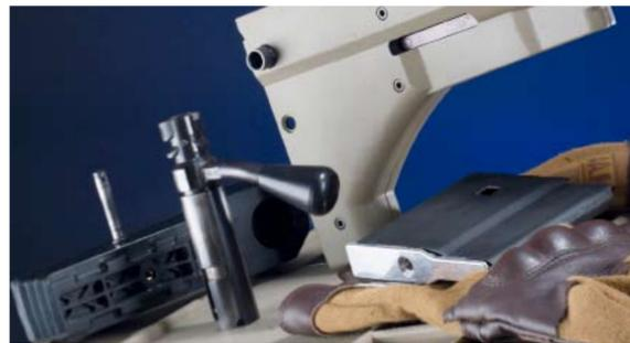
**Bolt can be removed for maintenance or caliber change by just pressing a pin, sliding off butt plate and pulling bolt out of the rifle's stock/receiver assembly.**
