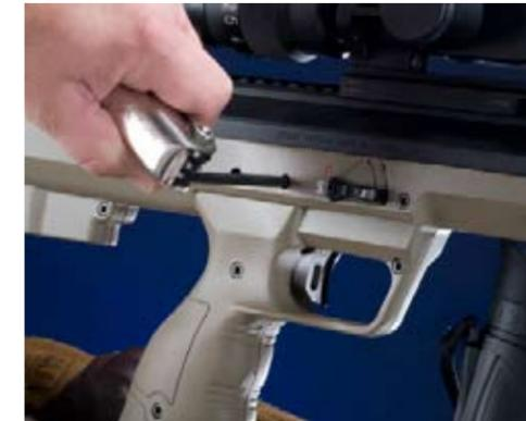
**Barrel is removed by turning three retaining bolts a half turn and then sliding barrel out the front of the stock/receiver assembly.**
